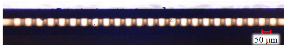
Fig. 4. Cross section of a GI square-core waveguide.
